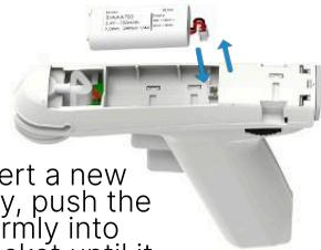
To insert a new battery, push the plug firmly into the socket until it snaps into place.
